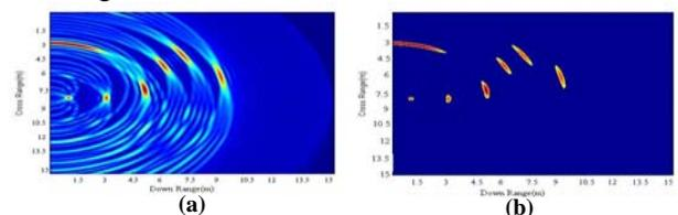
Figure 6. Results of backprojection algorithm (a) raw image (b) image after thresholding
