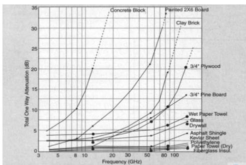
Figure 2. Illustrating through-wall EM attenuation<sup>[9]</sup>
