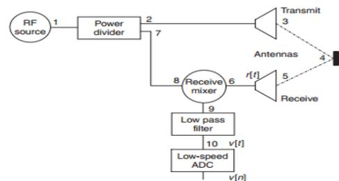
Figure 4. Homodyne Architecture for SFCW Processing
