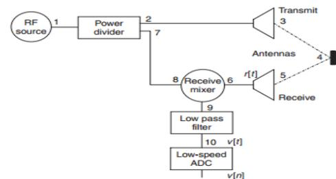
Figure 4. Homodyne Architecture for SFCW Processing
