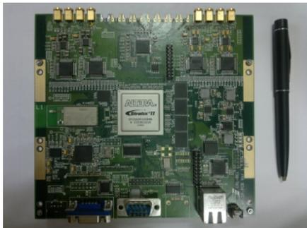
Figure 8. Multi-channel signal processing hardware
