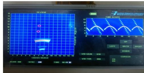
Figure 9. A view of TWR user display showing 2-D display (left) and time scope (right)
