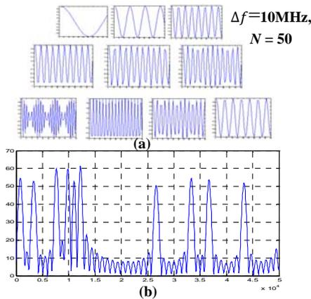
Figure 5. (a) Simulated SFCW baseband sampled echo from 10 scatterers and (b) composite range profile of targets
