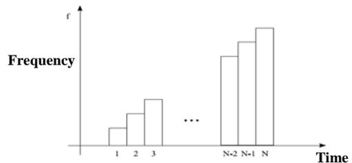
Figure 3. Transmitted signal frequency profile
