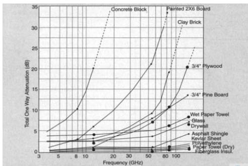
Figure 2. Illustrating through-wall EM attenuation<sup>[9]</sup>
