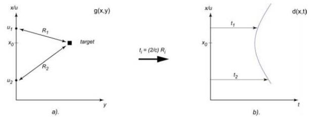
Figure 6. Transformation from object space to data space. Radar-to-target distance converted to round-trip return times.
