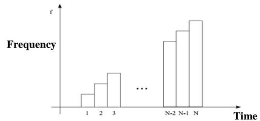
Figure 3. Transmitted signal frequency profile
